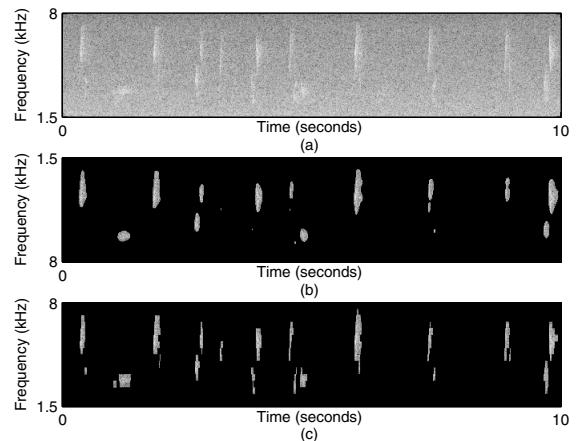
**Fig. 1.** Spectrograms of audio clip with id 2. Best viewed on a computer monitor. (a) Original spectrogram. (b) Segmented spectrogram (by [2]). (c) Segmented spectrogram (ours). Notice the faint signals detected by our algorithm.
