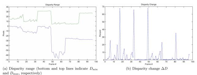
Figure 4. Disparity range (a) and change (b) for the IVC 3D image sequence (the picture changes every 16 frames).
