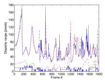
Figure 3. Disparity range for New Tsukuba Stereo Dataset sequence (dashed/red: ground truth, solid/blue: estimate).
